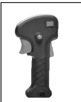
6. When the engine is running and idling. The throttle lever on handle is as above picture. First press the lock off lever and then switch the throttle lever on, the machine will be working.
